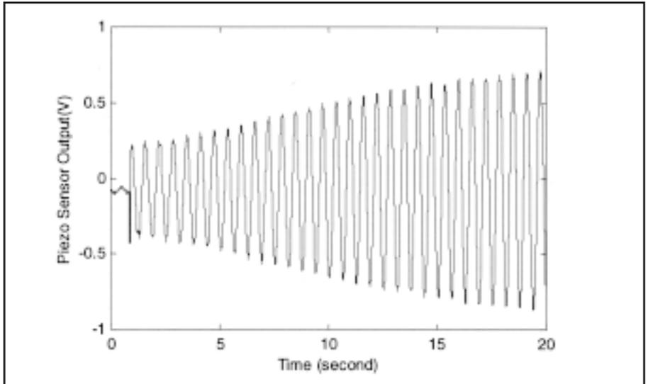
**Figure 7. Resonance of the flexible beam near its first modal frequency**
