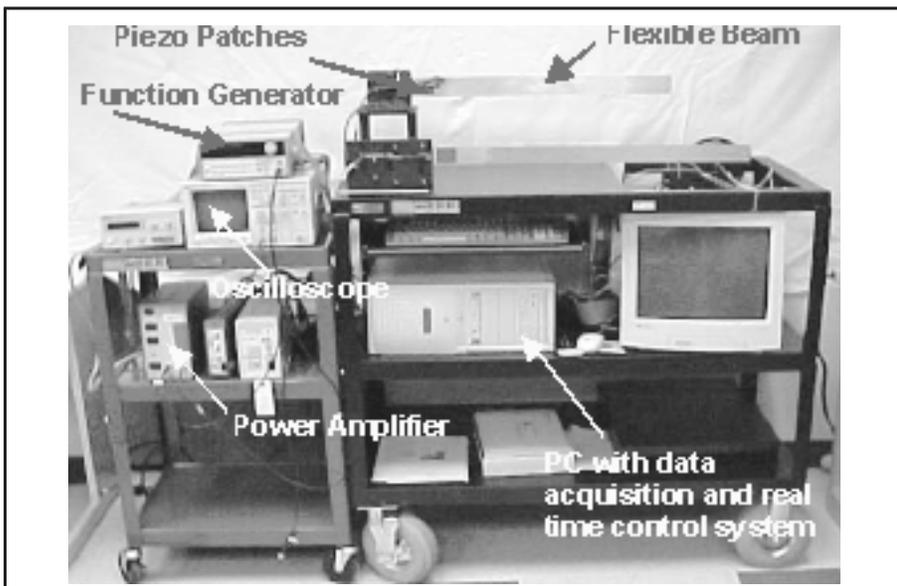
**Figure 5. The flexible beam setup which can be brought to classroom**
