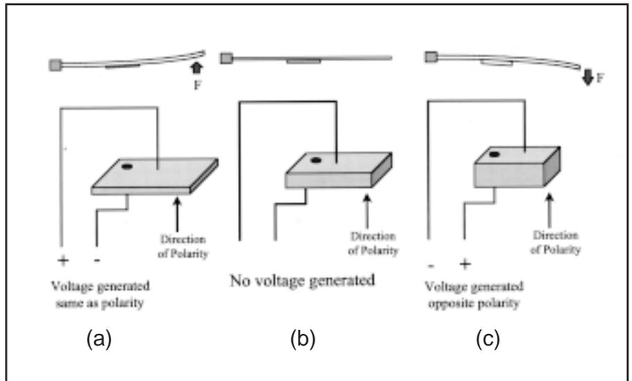
**Figure 3. Piezoceramic Patch as a Sensor**
