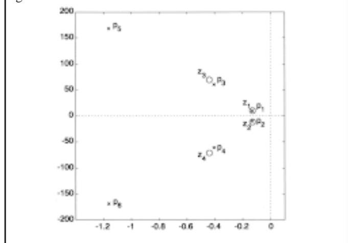
Figure 9. Zero and pole configuration of the flexible beam
