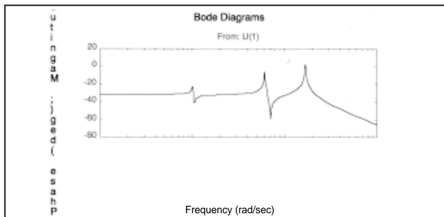
Figure 11. Bode diagram of the flexible beam
