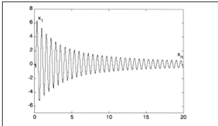
**Figure 6 Free response of the flexible beam vibration at its 1<sup>st</sup> mode**
