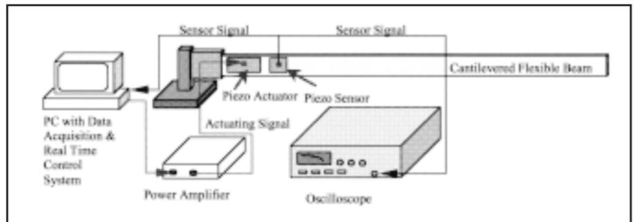
**Figure 4. Cantilevered flexible Beam with Piezo Sensor and Actuators**
