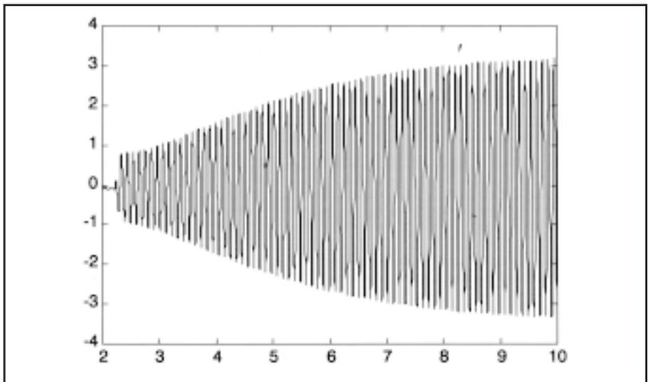
**Figure 8. Resonance of the flexible beam near its second modal frequency**
