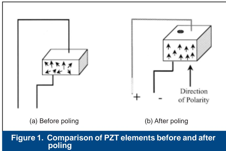
crystalline ceramics are ferroelectric materials with the perovskite crystal structure such as barium titanate and lead zirconate titanate (PZT). Ferroelectric ceramics become piezoelectric when poled. Lead zirconate titanate ceramics (PZT) and their modifications are solid solutions of lead titanate and lead zirconate.
