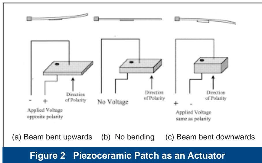
compare to Figure 2(b) when no voltage is applied. Now the polarity of the applied voltage is reversed, and the PZT patch shrinks laterally and bends the beam downwards (Figure 2(c)). These are examples of motor or actuator action, the conversion of electrical energy into mechanical energy. Finally, if an alternating voltage is applied to the electrodes, the cylinder will grow and shrink at the same frequency as that of the applied voltage. This will cause the beam to vibrate.
